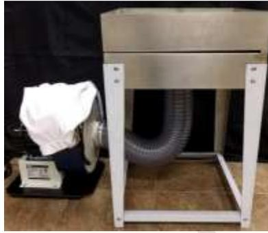
**CocoaT Max cooling Tray** – Top tray doubles as collection tray for the roasted beans in the roaster. Available in 110V or 220V. Place the top tray in the CocoaT commercial Roaster after roasting is done. Release the latch in the roaster drum. All the beans are collected in the top collection tray. Then remove the tray from the roaster and place it on the cooling mechanism and switch on the power. All the beans are cooled in less than 5 minutes.
