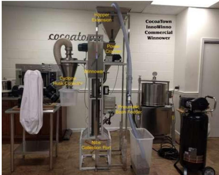
InnoWinno Winnower is a high efficiency, high throughput compact system that separates husk from the cracked cocoa beans to yield clean nibs. This system is cheaper, compact, dust free and more efficient than the models available in the market.
