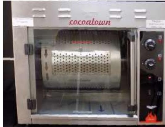
CocoaT commercial Roaster is a heavy duty Stainless steel roaster. The unit comes with roasting drum that can roast up to 20 lbs of cocoa beans in a single batch. The temperature and timer control lets the user customize it depending on the cocoa beans used.
